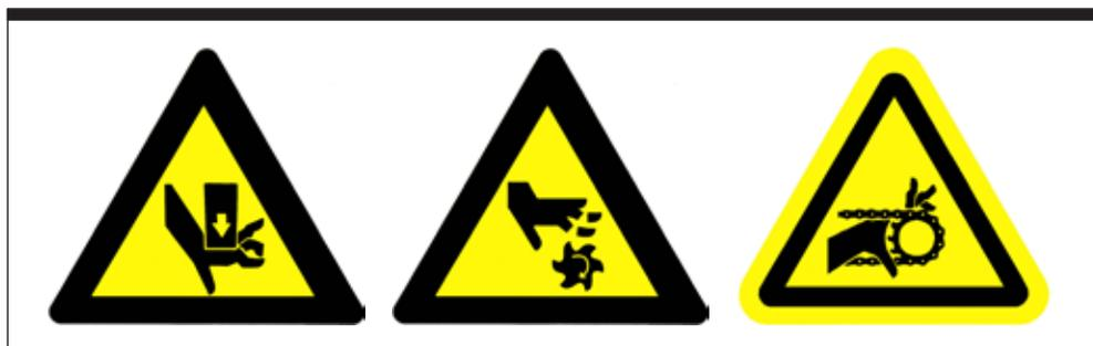
Figure 2-1. Additional Safety Warning Labels - Hand Crush, Finger Cut, Hand in Gears.
