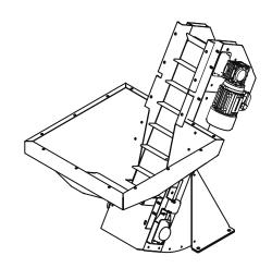
The Shibuya Hoppmann ET-02 Elevating Table Top Prefeeder is designed to handle a variety of small sized, light weight parts with both an adjustable base and head chute to accommodate small product loading and delivery variances. The concept is based on the standard sized elevating prefeeders but has a more compact footprint and is designed to be mounted on top of an existing support table.
